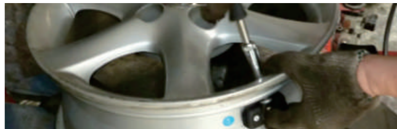
Well fitted Internal Sensor
