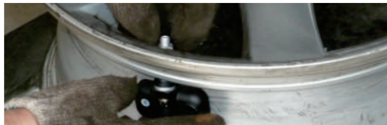
Well fitted Internal Sensor
