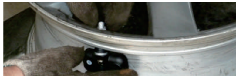
Well fitted Internal Sensor
